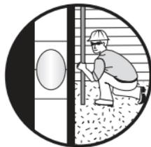
View through instrument in level position showing bubble centered on center mark.
